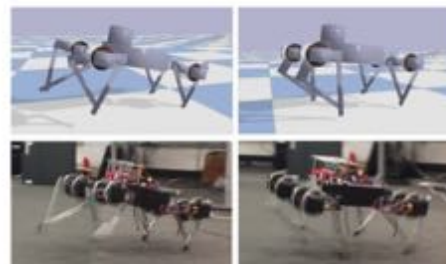
Fig. 1: The simulated and the real Minitaurs learned to gallop using deep reinforcement learning.
